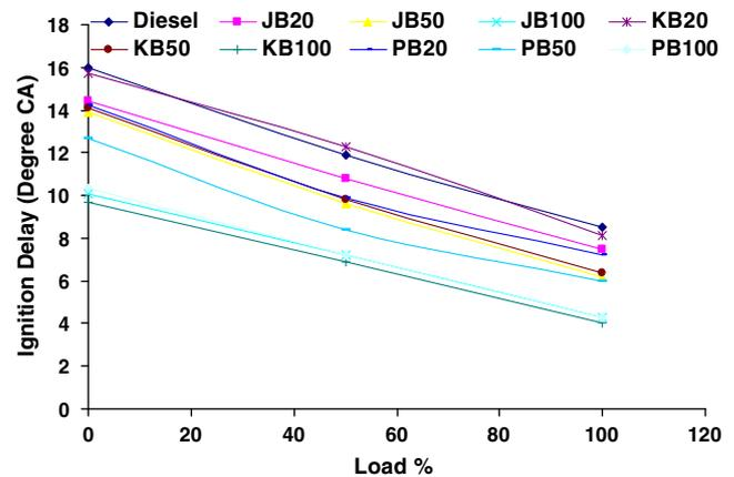
Fig. 4. Effect of load on the ignition delay for diesel, biodiesel and their blends.
