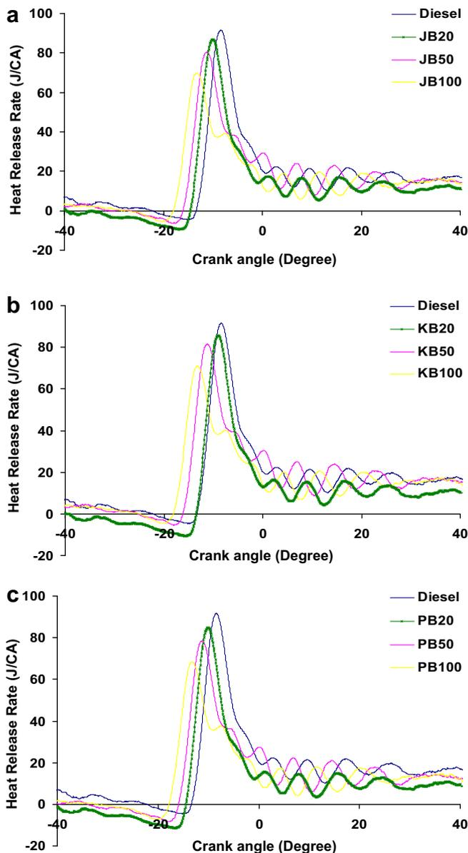
Fig. 3. (a) Heat release rate for diesel, Jatropha biodiesel and blends at full load. (b) Heat release rate for diesel, Karanja biodiesel and blends at full load. (c) Heat release rate for diesel, Polanga biodiesel and blends at full load.
