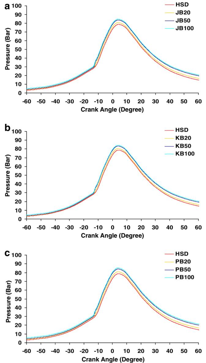
Fig. 2. (a) Pressure vs. crank angle for diesel, Jatropha biodiesel and blends at full load. (b) Pressure vs. crank angle for diesel, Karanja biodiesel and blends at full load. (c) Pressure vs. crank angle for diesel, Polanga biodiesel and blends at full load.
