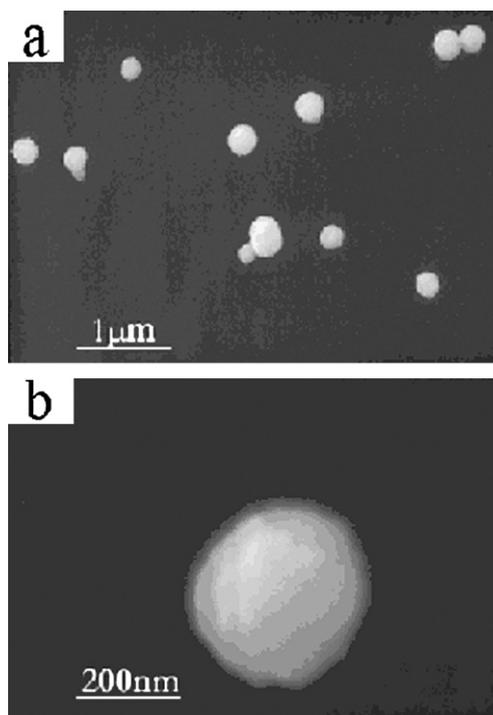
Fig. 4 SEM photographs of (a) monodisperse silver particles and (b) a single silver particle.
