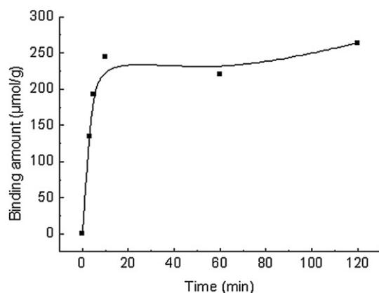
**Fig. 8** Kinetic binding profile of testosterone binding to the imprinted Ag-Si particles. The imprinted particles used here were prepared with a reaction time of 24 h.
