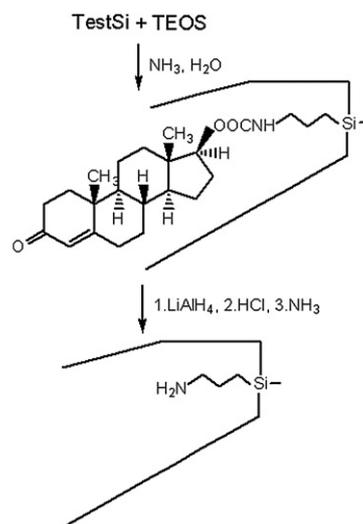
Fig. 2 Schematic synthesis route for testosterone–imprinted silica films.
