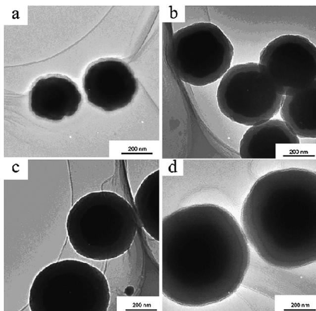
**Fig. 5** HRTEM images of the silver particles coated with testosterone-imprinted silica films synthesized (a) with a reaction time of 12 h, (b) repeating reaction twice, (c) repeating reaction thrice, and (d) repeating reaction four times.
