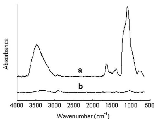
**Fig. 6** FT-IR spectra of (a) the silver particles coated with testosterone-imprinted silica film and (b) the blank silver particles.
