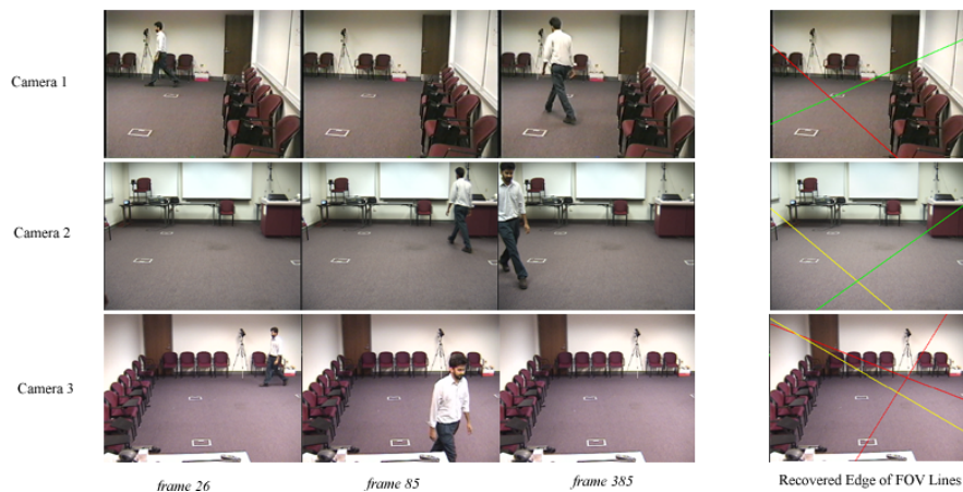
Figure 5: Determination of Edge of FOV lines using a short sequence of person walking in the room. The first 3 columns show triplets of sample images taken at same time instant. The last column shows the recovered lines
