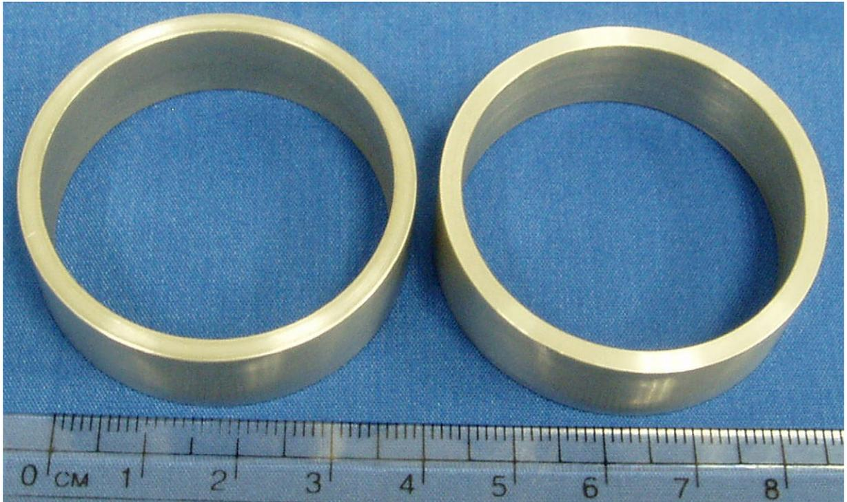
Fig. 122. HVOF spray formed hypereutectic Al-Si nanocomposite ring structures (3.85 cm inner diameter with a thickness of 2.5 mm) [348].
