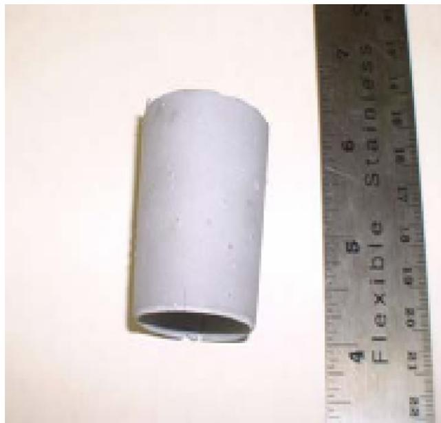
Fig. 118. Cylindrical-shaped alumina-Ni nanocomposite structure with 1.2 in. outer diameter, 1 in. inner diameter, and 1.5 in. length [345].
