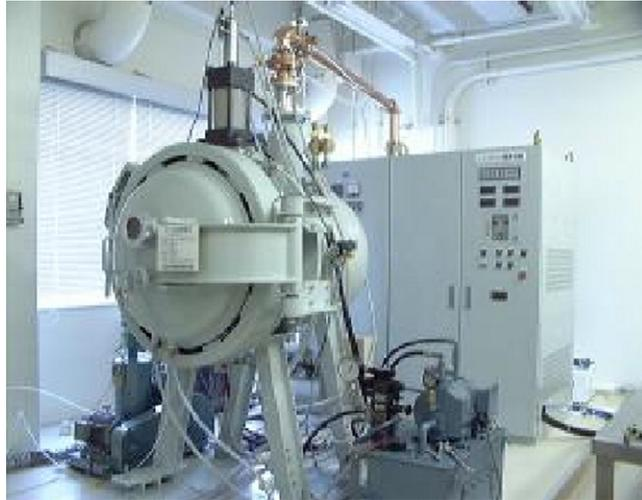
Fig. 89. Microwave sintering system with attached press. (Source: [www.ifs.tohoku.ac.jp/divisions/en/ifsd\\_isl.html](http://www.ifs.tohoku.ac.jp/divisions/en/ifsd_isl.html).)
