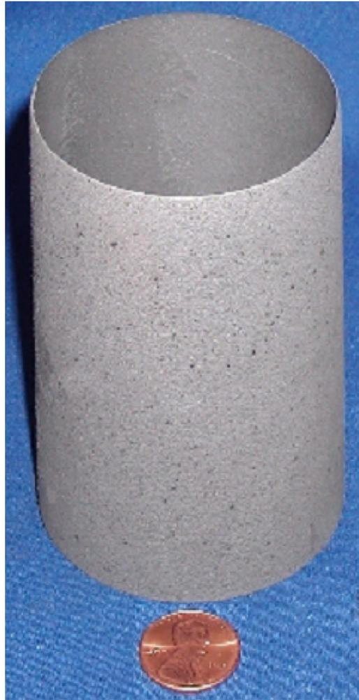
Fig. 109. Plasma spray formed hollow cone-shaped Al–CNT composite structure [335].
