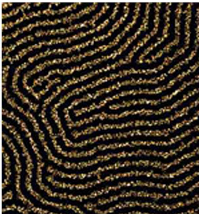
Fig. 196. Nanoparticles and nanowire arrays templated by a stripe pattern formed at the surface of a polystyrene–PMMA di-block copolymer by vapor deposition of gold. (Source: <http://magazine.uchicago.edu/0212/features.>)
