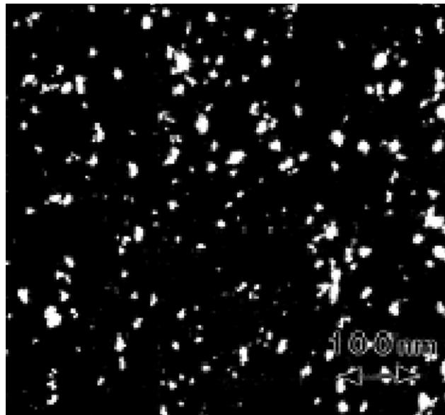
Fig. 184. TEM microstructure of nanocrystalline Ni with an average grain size of 11 nm. (Reproduced with permission from Elsevier from [447].)
