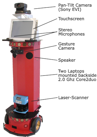
Fig. 2. Hardware composition of BIRON: It is equipped with several sensors that allow perception of the current situation as a basis for interaction. Feedback is provided by speech synthesis and using a virtual character displayed on the touchscreen. The robot's on-board computational equipment in combination with a wireless LAN notebook is sufficient to achieve a system running responsive enough for fluent HRI.
