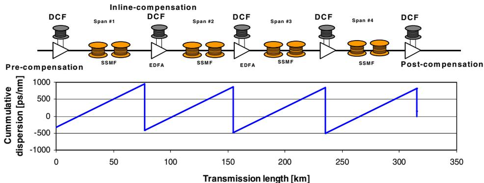
Fig. 3: Dispersion map of the 107 Gbit/s NRZ transmission experiment
