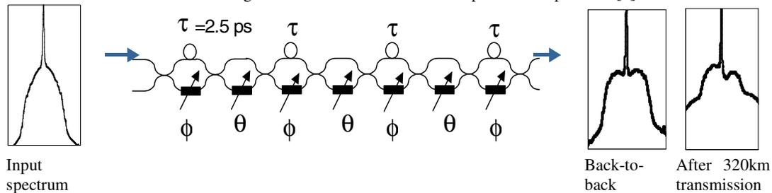
Fig. 2: Schematic of the PLC Equalizer together with optical input and output spectra
