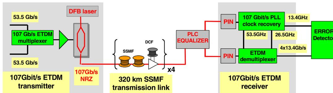
Fig. 1: Schematic setup of the 107 Gbit/s ETDM transmission experiment
