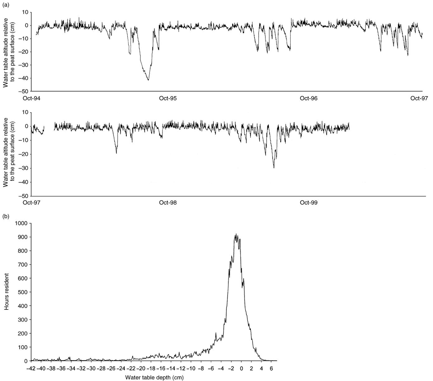
**Fig. 3** Hourly water table depth, cm, at the ECN target dipwell. (a) Time-series. (b) Water table residence curve.
