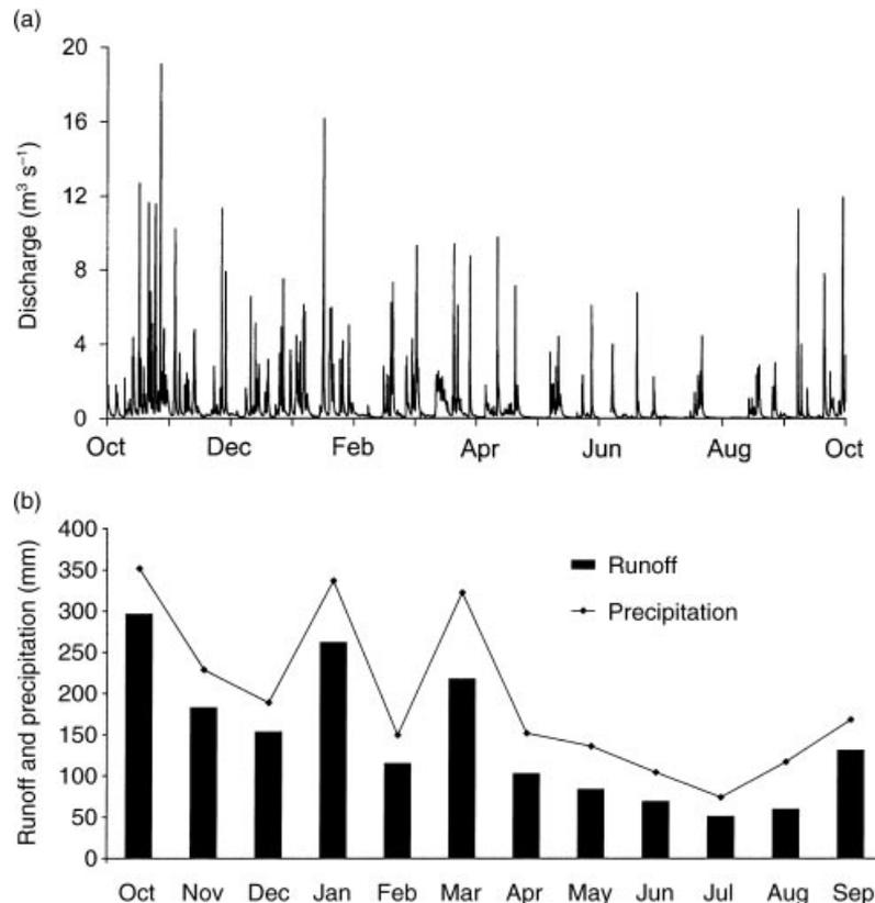
Fig. 2 Discharge from Trout Beck during the 1999 water year. (a) 15 minute readings. (b) Monthly rainfall and runoff totals.
