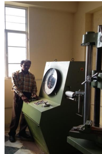
Figure- Universal Testing Machine With Plotter & Hydraulic Load Dial
