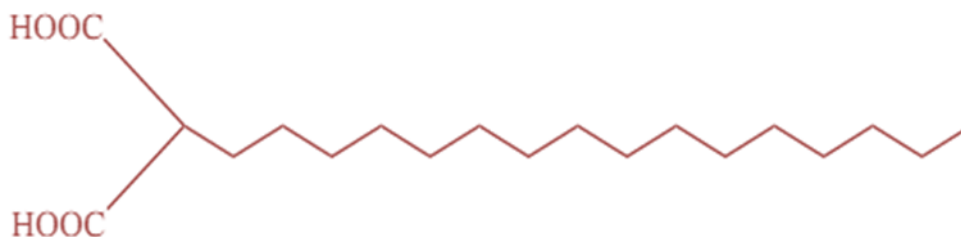
Fig. 6 Molecules of hexadecylmalonic acid (HDMA) used for the surface modification in QDSSC
