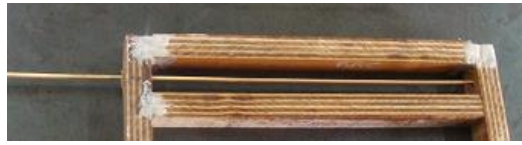
Figure 3: Mould for single fiber pull-out test
