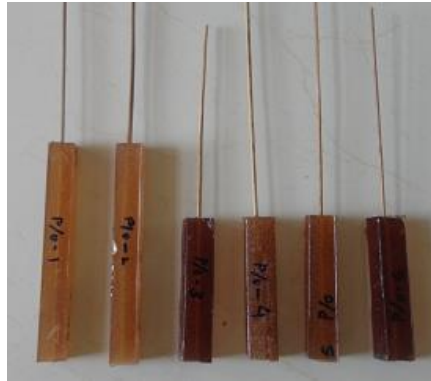
Figure 4: Specimens for single fiber pull-out test
