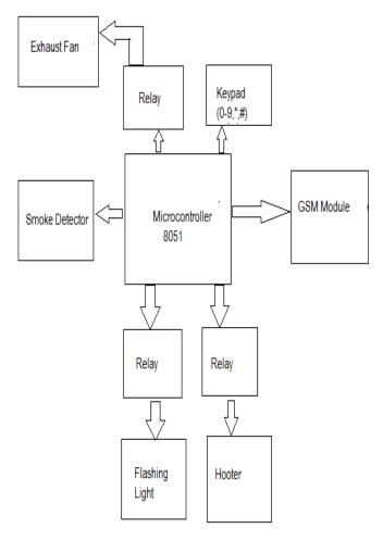
Fig. 4. Block diagram for fire and smoke detection
