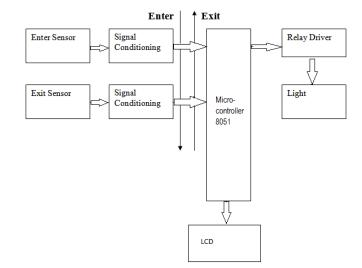
Fig.2. Block diagram for automatic light switching
