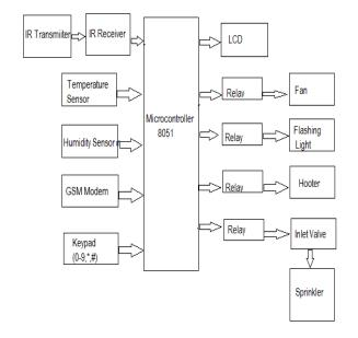
Fig.1. Block diagram for integrated system
