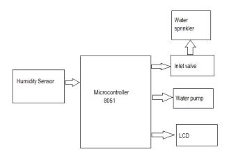
Fig. 7. Block diagram for in-house sprinkler system
