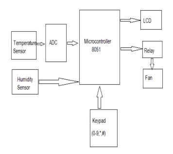
Fig. 3. Block diagram for climate control
