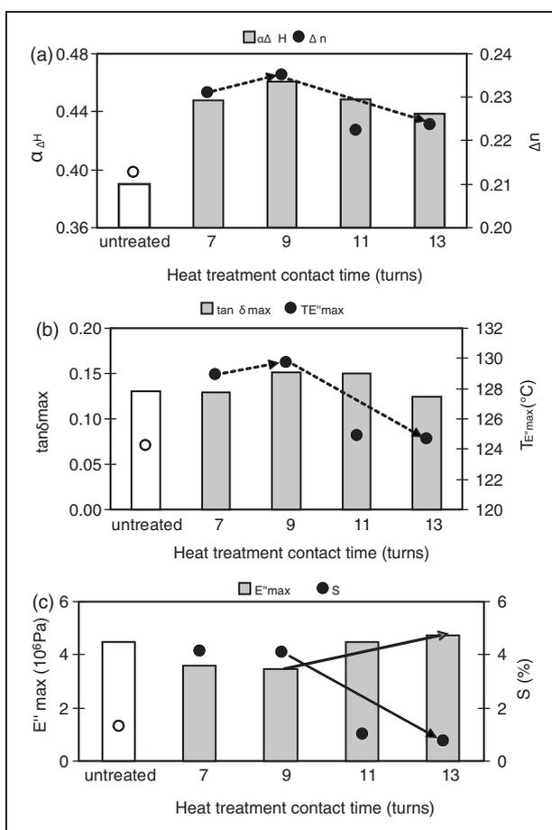
**Figure 2.** Influence of the heat treatment contact time on structural parameters. Threads were treated at constant temperature of 200 $^{\circ}$ C on the second heated cylinder. (a) degree of crystallinity/birefringence, (b) loss tangent/temperature of the loss modulus, (c) loss modulus/shrinkage.
