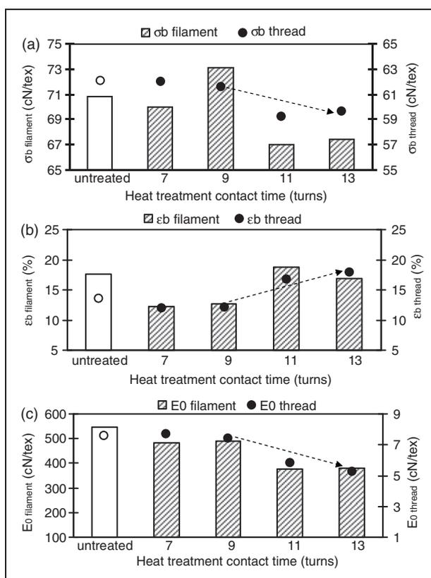
**Figure 4.** Influence of the heat treatment contact time on mechanical properties. Threads were treated at constant temperature of 200°C on the second heated cylinder. (a) breaking tenacity, (b) breaking extension, (c) elastic modulus.
