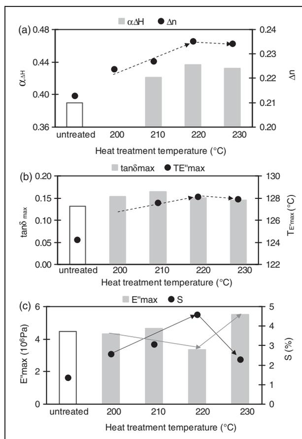
**Figure 1.** Influence of the heat treatment temperature on structural parameters. Threads were treated at constant contact time of 5 turns on the second heated cylinder. (a) degree of crystallinity/birefringence, (b) loss tangent/temperature of the loss modulus, (c) loss modulus/shrinkage.
