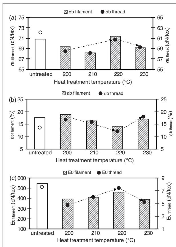
**Figure 3.** Influence of the heat treatment temperature on mechanical properties. Threads were treated at constant contact time of 5 turns on the second heated cylinder. (a) breaking tenacity, (b) breaking extension, (c) elastic modulus.
