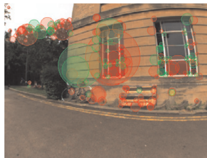
Fig. 12. Some examples of situations where the Chow Liu approximation outperforms naive Bayes. In (a), a change in lighting means that the feature detector does not fire on the windows of the building. In (b), the people are no longer present. In (c), the foreground text and the scaffolding in the top right are not present in the second image. In each of these cases, the missing features are known to be correlated by the Chow Liu approximation, hence the more accurate probability. Words common to both images are shown in green, others in red. The probability that the two images come from the same place (according to both the Chow Liu and naive Bayes models) is indicated between the pairs.
