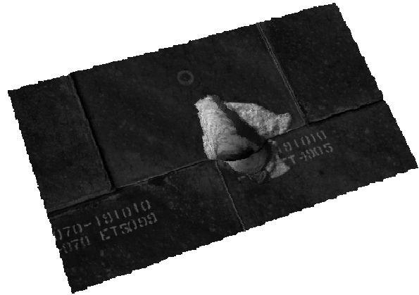
Figure 3 - LCS image of shuttle tile damage 3
