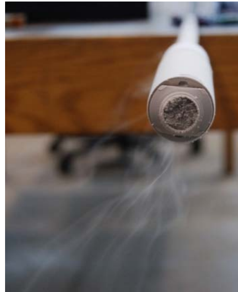
Figure 5 - Core capture mechanism after test at 90 Kelvin 5
