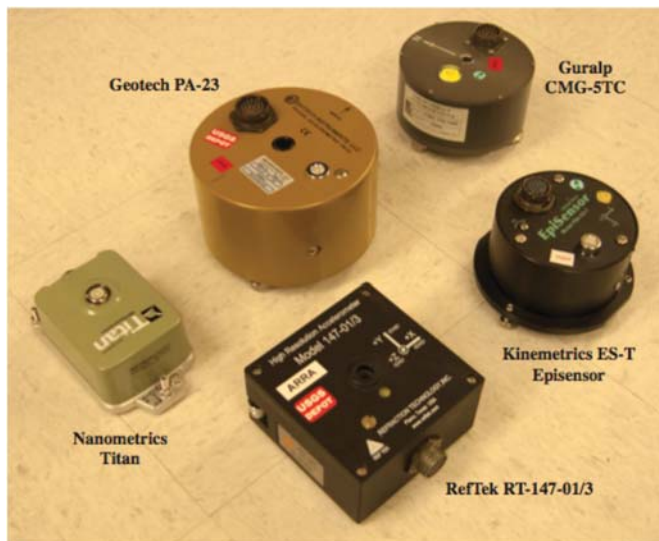
▲ Figure 1. Examples of the strong-motion accelerometers used in this test. The Kinemetrics EpiSensor ES-T has the same case as the Kinemetrics EpiSensor ES-T Nickel (not shown). Each tile is approximately 0.3 m.
