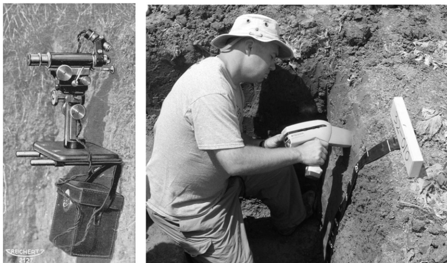
Fig. 1. Two examples from in-situ observations and measurement in a soil pit. Left picture: Soil microscope with cross-slide stand attached to the wall of a soil pit; the leather box stores the battery for the oblique illuminator, from Kubišna (1938). Right picture: portable XRF to determine contaminant metal depth migration in a soil profile (picture from David Weindorf).
