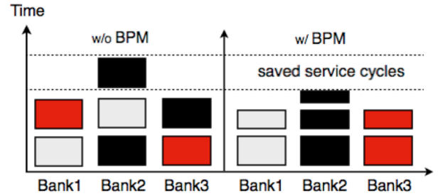
Figure 2. The Comparison between interleaved address mapping and BPM. Different colors mean that the requests are from different threads.
