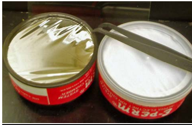
Figure 7.1: Electret ion chambers used for measurement of radon and thoron progeny deposited on the surface.
