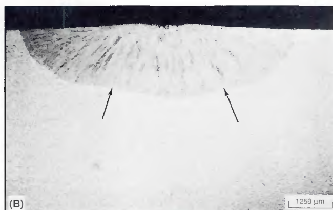
Fig. 1—Transverse macrograph of the GTA weld indicating the fusion zone shape and size (Heat A containing 90 ppm sulfur). A—After 2 s; B—after 5 s. Arrows indicate inflection in the fusion zone geometry.
