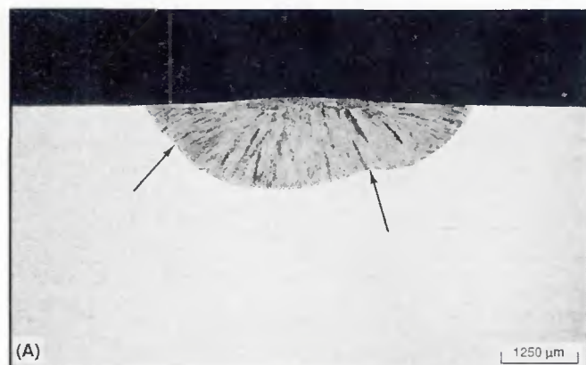
Fig. 1—Transverse macrograph of the GTA weld indicating the fusion zone shape and size (Heat A containing 90 ppm sulfur). A—After 2 s; B—after 5 s. Arrows indicate inflection in the fusion zone geometry.
