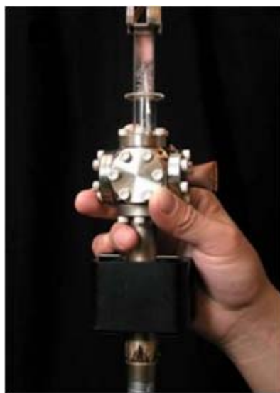
Figure A2.1: Miniature atom-chip vacuum cell with a 2 L/s ion pump.
