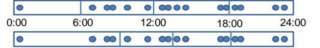
Figure 1: Equal width discretization (top) would result in more natural boundaries. Equal frequency discretization (bottom) would use bins more efficiently and prevent too few samples in some bins.
