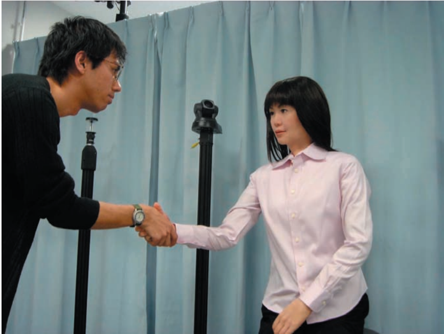
Figure 5. Repliee Q2 (“Uando”) is controlled by air actuators that provide 43 degrees of freedom. The android can make facial expressions, eye, head, and body movements, and gestures with the arms and hands. Touch sensors with sensitivity to variable pressures are mounted under her clothing and silicone skin. Repliee Q2 uses floor sensors and omnidirectional vision sensors to recognize where people are in order to make eye contact while addressing them during conversation. Repliee’s interactions are largely scripted, but she can respond to the content and prosody of her interaction partner by varying what she says and the pitch of her voice.
