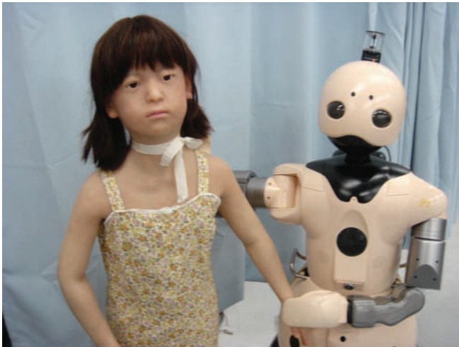
Figure 1. Hiroshi Ishiguro's Intelligent Robotics Laboratory at Osaka University developed the two robots shown above, the android on the left named Repliee R1, a joint effort with Kokoro Co., Ltd., and the humanoid on the right named Eveliee P1, a joint effort with Mitsubishi Heavy Industries.
