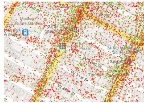
Fig. 5. Estimated WiFi AP locations in a 0.4x0.5 sq.mile area in Manhattan, NY. Red dots indicate single citation in the crowd sourced war-driving database. Green dots indicate multiple citations. Source:WiGLE [9]
