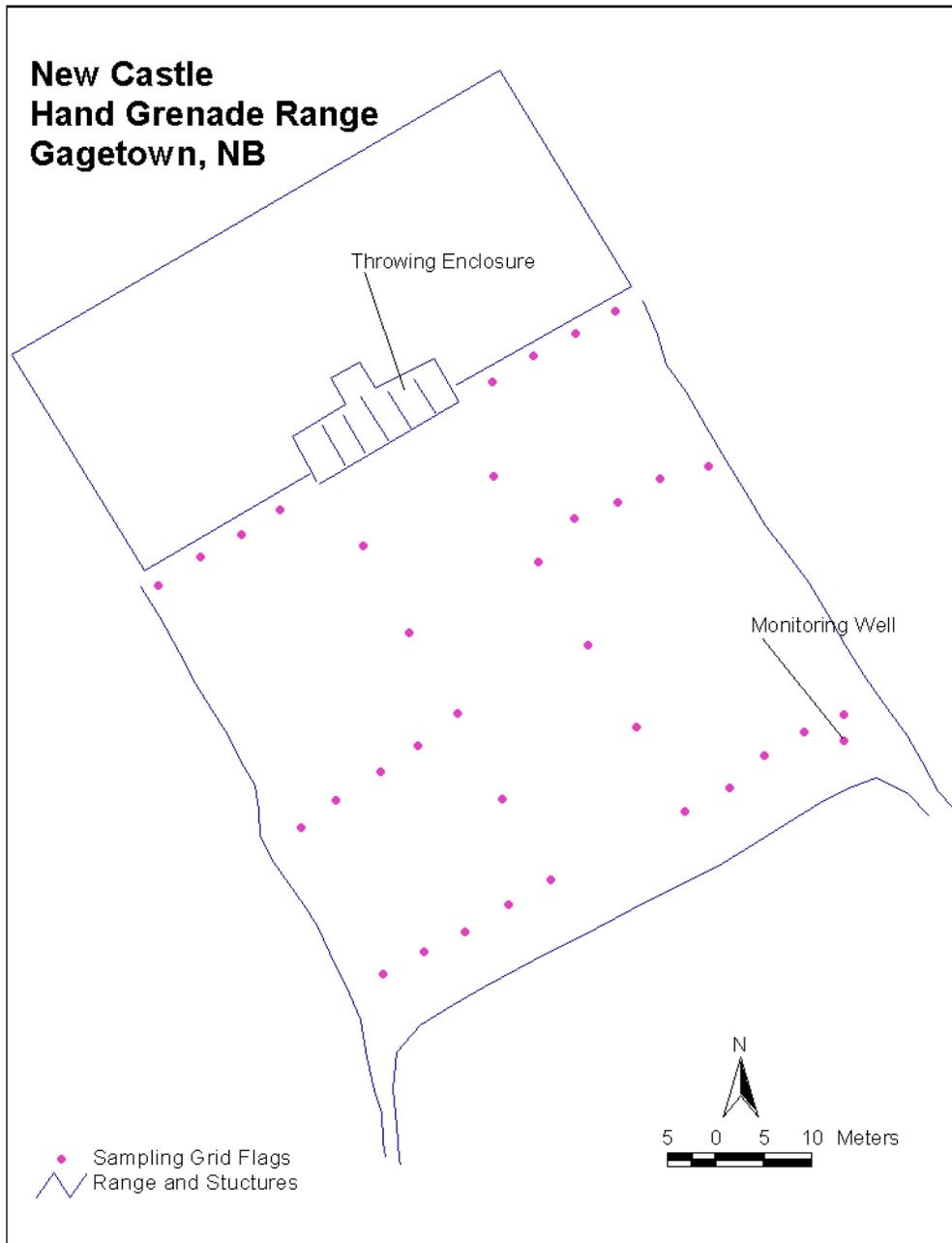
**Figure 14. New Castle Hand grenade range sampling pattern**
