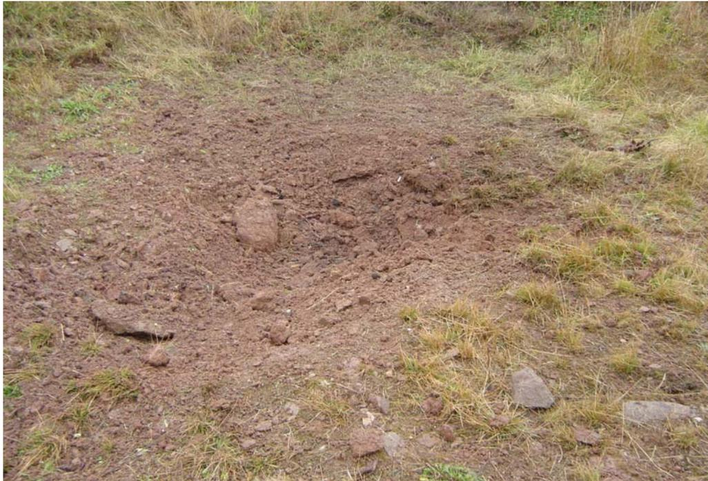
**Figure 10. Crater formed after the blow in place of 84 mm HEAT round**
