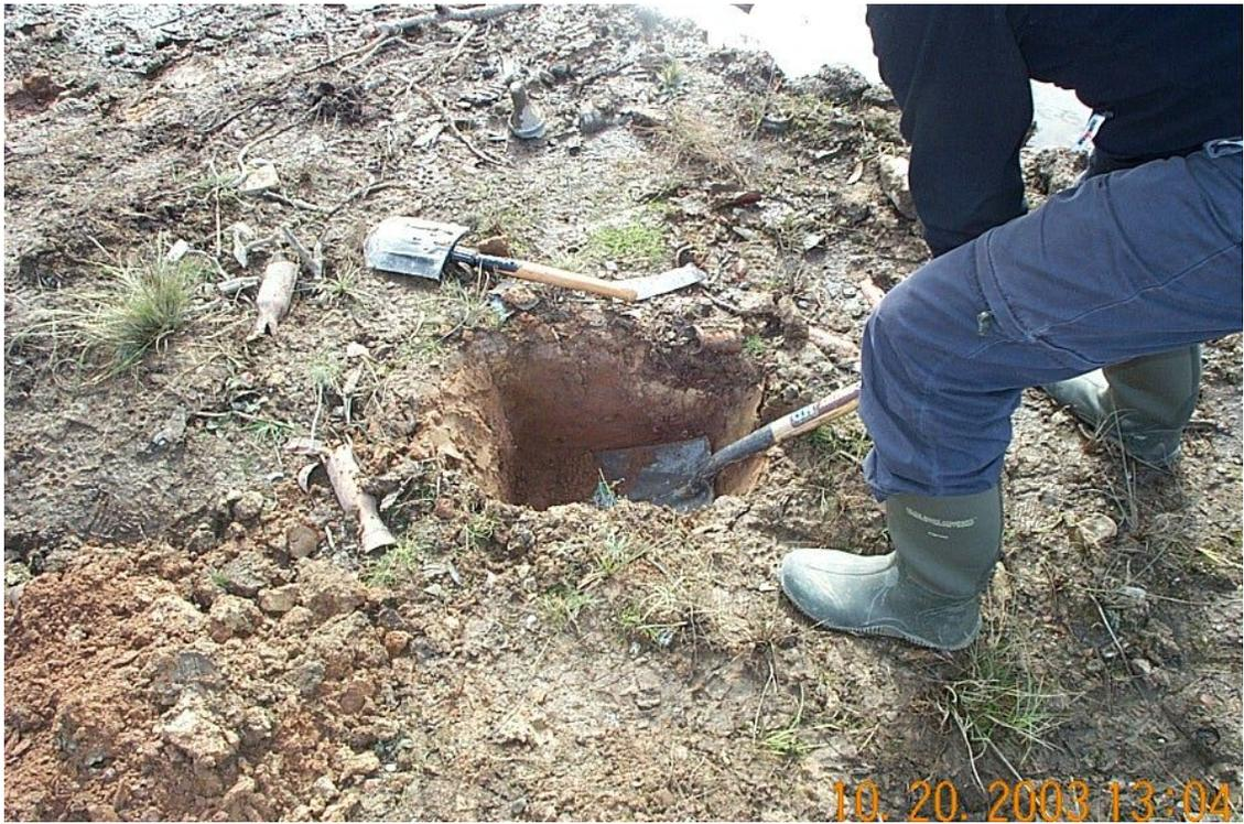
**Figure 6. Digging for depth sampling profiling**
