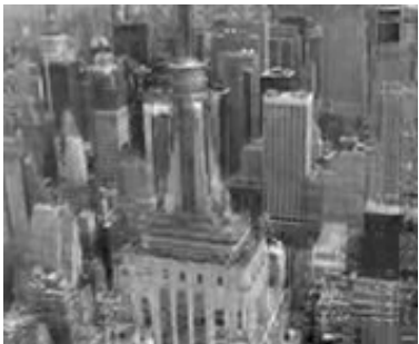
(c) Image in frame buffer computed using DCT with a faulty PE 2 , PSNR=29.86dB
