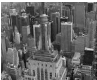
(d) Image in frame buffer computed using DCT with a faulty PE 7 , PSNR=34.78dB
