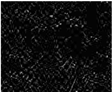
(b) Image in frame buffer computed using DCT with a faulty PE 1 , PSNR=7.07dB
