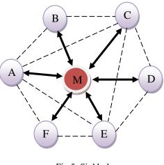
Fig 5: Sinkhole Attack
