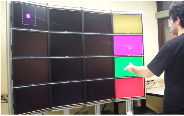
Figure 4: Prototype overview. This photograph depicts a user interacting with the two legs of LOP-cursor. Notice that while leg-1 selects a square on the left, the leg-2 ring indicates the location on the right to where the square will be moved.
