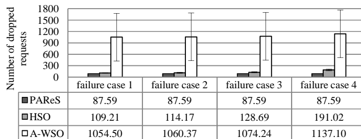
Fig. 11. The average number of persistent-update-operation requests dropped during the service downtimes of the PAREs, HSO, and A-WSO on different failure cases.
