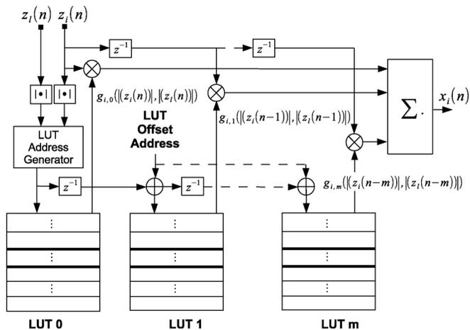
Fig. 4. Block diagram of the 2D-DPD LUT implementation.
