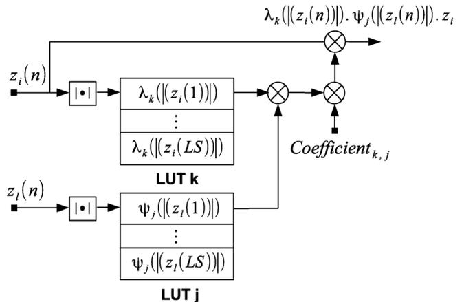
Fig. 5. Block diagram of 2D-DPD basic cell.
