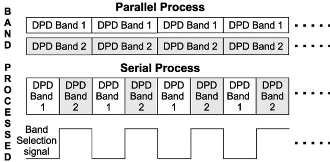
Fig. 6. Time sequence view of the band operations.
