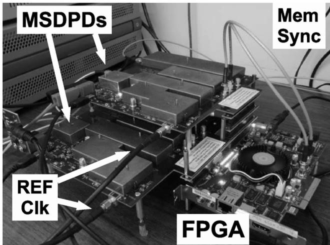
Fig. 9. FPGA and MSDPDs configuration for dual-band DPD.
