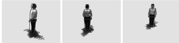
Fig. 5. Appearance model acquisition. Three pictures are taken for each target, sampling a front, side and back view. Foreground blobs are extracted by background suppression and morphological noise cleaning. Head position is estimated by triangulation, and target height is derived. Projected shape identifies blob parts from which head-torso-legs histograms are extracted.
