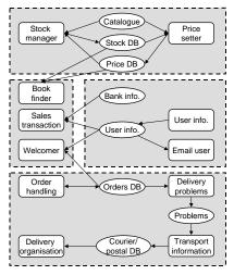
In order to evaluate a potential grouping for coupling we use an *agent acquaintance diagram*. This diagram simply links each agent with each other agent with which it interacts. A design with fewer linkages is less highly coupled and therefore preferable.
