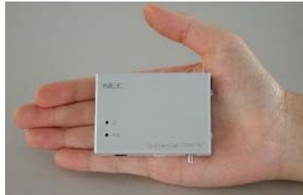
(b) Photo of encapsulated transceiver module
