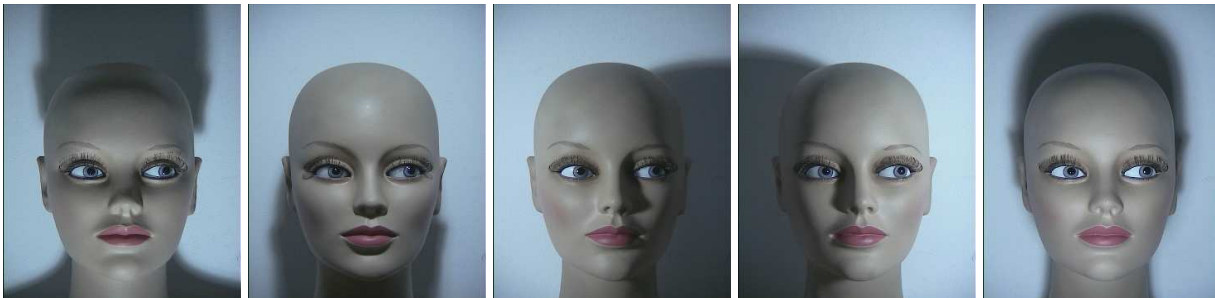
Figure 2: The input images for the shape from stereo reconstruction process. Same camera position and head object with different lighting directions.
