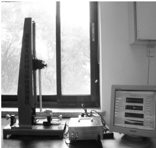
Figure 3. Cantilever beam tester for thin wood composite
