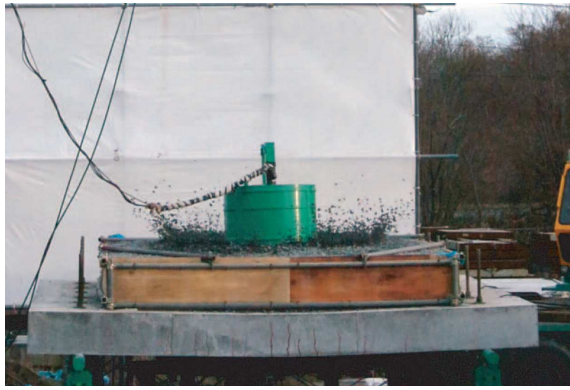
Fig 1: Falling weight impact test [3]
