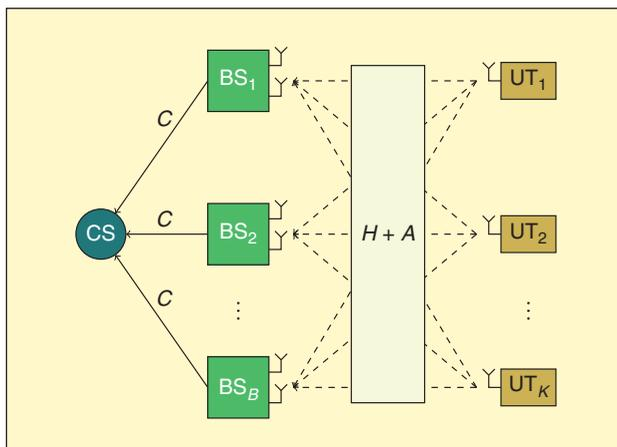
FIGURE 2 Virtual cell uplink channel.
