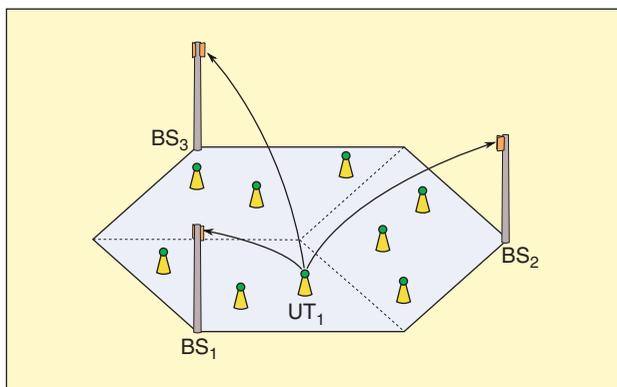
FIGURE 3 Virtual cell with three BSs serving nine UTs.
