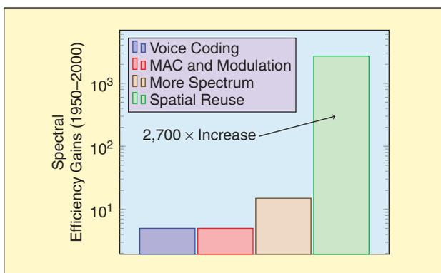
**FIGURE 1** Sources of spectral efficiency gains of wireless communication systems from 1950 to 2000 [3].
