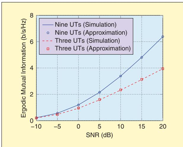
**FIGURE 4** Normalized ergodic mutual information versus transmit SNR for different numbers of UTs.
