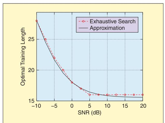
**FIGURE 6** Optimal training length versus transmit SNR for a coherence time of 100 channel uses.
