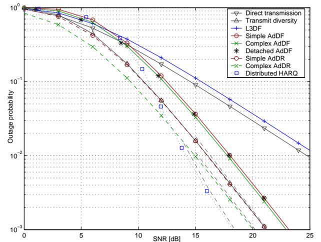
Fig. 2. Performance of the different conventional and cooperative relaying protocols in terms of outage probability versus SNR for spectral efficiency  $R=2$  bit/channel use. Full second order diversity is achieved by all cooperative protocols.
