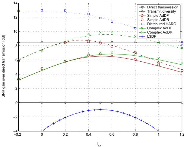
Fig. 3. SNR gain of different protocols over direct transmission.  $r_{s,r}$  denotes the position of the relay between source and destination, normalized to the source-destination distance. The maximum SNR gain for most cooperative protocols is obtained for  $r_{s,r} \approx 0.5$ . For the distributed Hybrid ARQ however, it is favorable to place the relay as close to the source as possible – to ensure an almost perfect source-relay channel.
