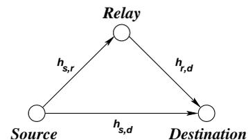
Fig. 1. Illustration of a cooperative relaying scenario. The source sends a broadcast message to destination and relay. The relay then forwards additional information about the source message to the destination, which appropriately combines the received data.
