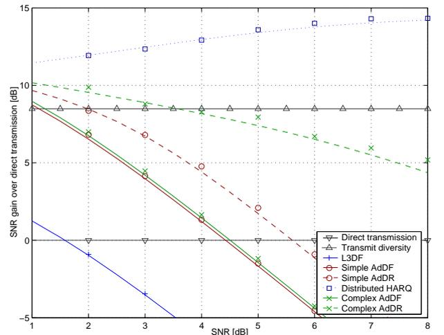
Fig. 4. SNR gain of different protocols over direct transmission as a function of the spectral efficiency  $R$ . The relay is located halfway between source and destination, i.e.,  $r_{s,r} = 0.5$ . Decode-and-Forward type protocols all lose 3dB per increase in spectral efficiency of 1 bit/channel use. Decode-and-Reencode protocols however, show more stable performance even as the transmission rate increases.
