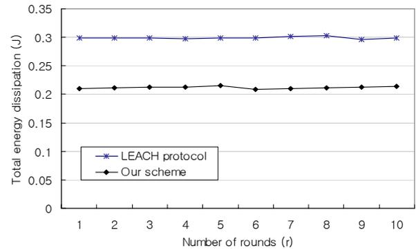
**Fig. 7.** Average of total Energy dissipation by our scheme and LEACH
