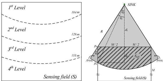
Fig. 2. Calculation of area ( $S_{sub}$ )
