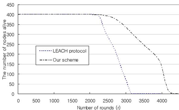
**Fig. 6.** System lifetime By our scheme and LEACH
