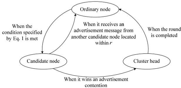
**Fig. 4.** State transition diagram of each sensor node
