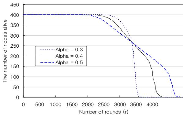
**Fig. 10.** System lifetime when alpha value is varied
