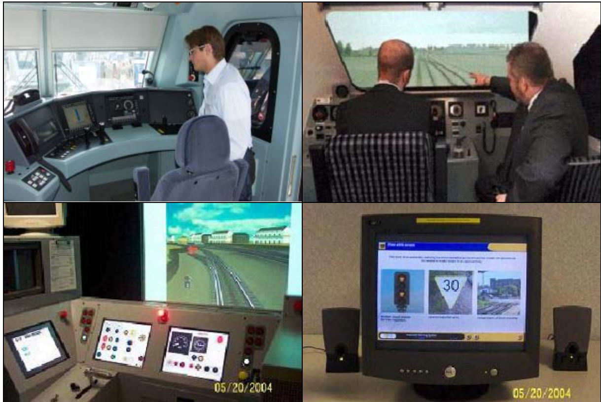
Figure 15: Different training tools: Real cab (top left), full simulator (top right), part task trainer (bottom left) and computer based training (bottom right) (top right and bottom: RSSB, 2005).
