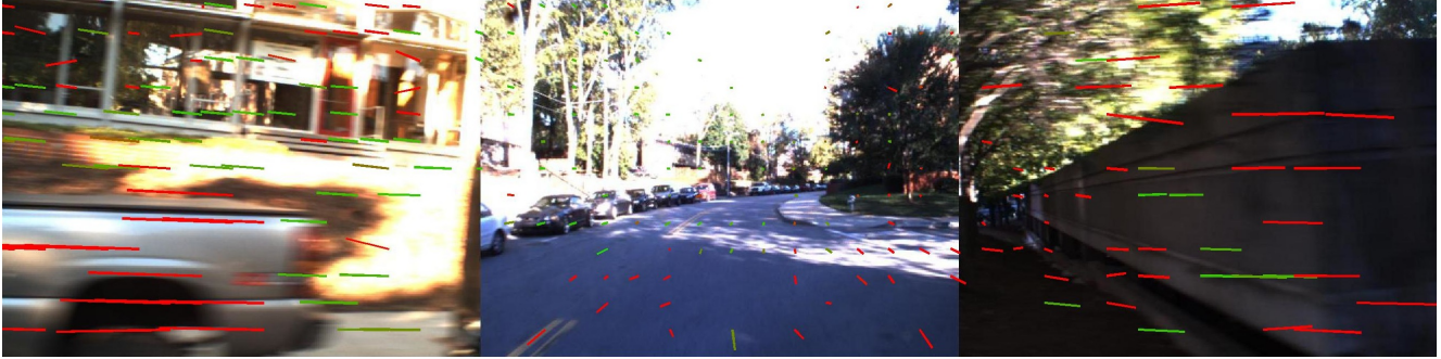
Figure 6: Detection of outliers in the sparse optical flow in a frame from the 3-camera outdoor driving sequence. Colored lines are sparse optical flow, ranging from green when p(\text{inlier}) = 1 , to red when p(\text{inlier}) = 0 . Sparse flow vectors that are inconsistent with the linear flow subspace have low inlier probability. Vectors on the moving pickup truck, in the textureless regions of the road, and on the very close and very far structure of the wall are labelled as outliers.
