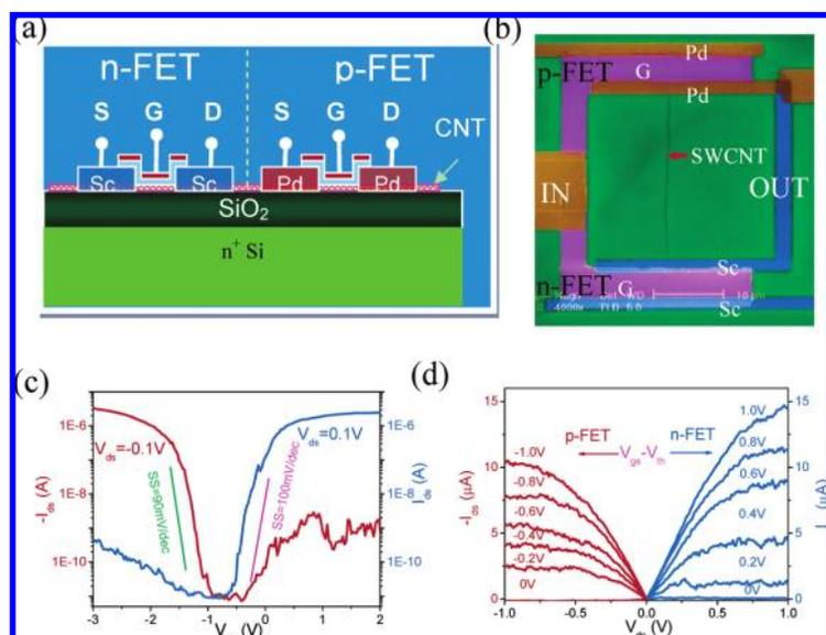
**Figure 1.** SWCNT-based CMOS FETs with self-aligned top gate. (a) Side view schematic of SWCNT CMOS devices with a pair of p- and n-FETs. (b) SEM image showing a SWCNT CMOS inverter which is composed of a p-FET (top) and an n-FET (bottom). The gate length for both FETs is 4  $\mu\text{m}$ . (c) Field transfer characteristics ( $I_{ds}-V_{gs}$ ) and (d) output characteristics ( $I_{ds}-V_{ds}$ ) of a pair of SWCNT CMOS FETs with gate length  $L_g = 1.0 \mu\text{m}$ .
