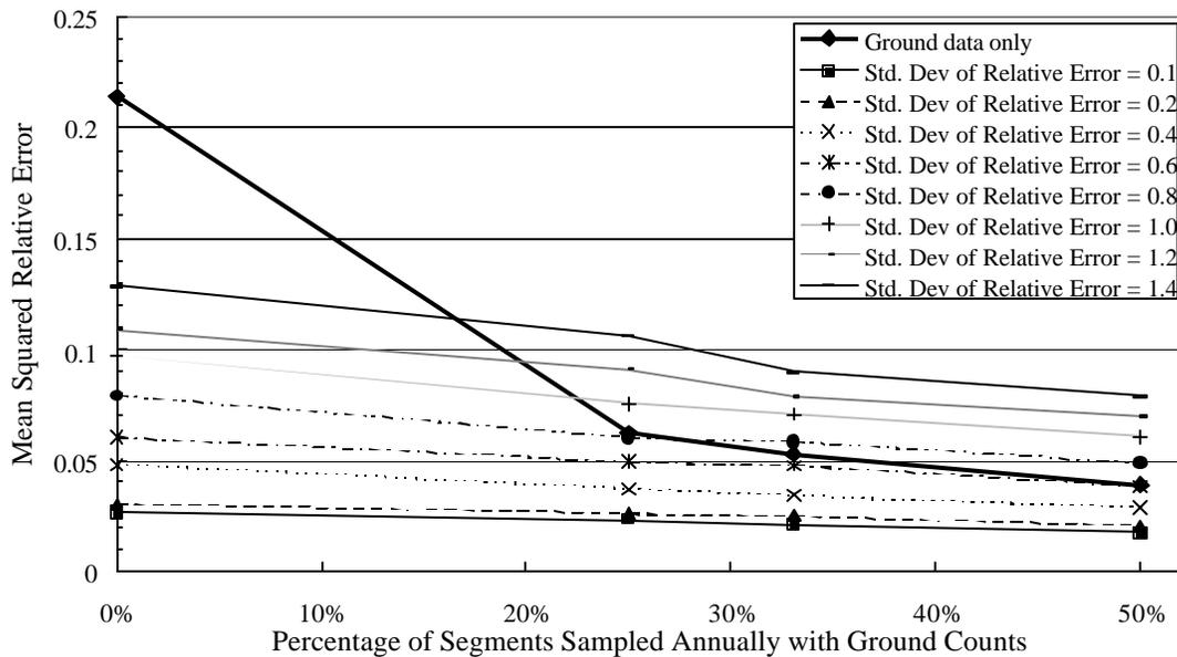
Figure 3b. Simulated mean-squared relative error in estimated VDT vs. percentage of highway segments sampled annually for different standard deviations of relative error of  $AADT^{img}$
