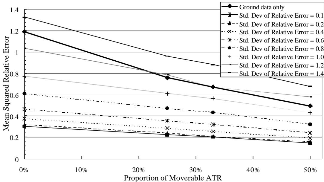
Figure 3a. Simulated mean-squared relative error in estimated AADT vs. percentage of highway segments sampled annually for different standard deviations of relative error of  $AADT^{img}$  (appears as Figure 2 in McCord, et al., (2002c))
