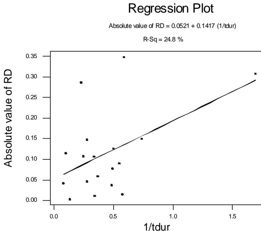
**Figure 2. Plot of empirical data and least squares fit of Absolute Value of Relative Difference ( $RD$ ) vs. ( $1/t^{dur}$ )**
