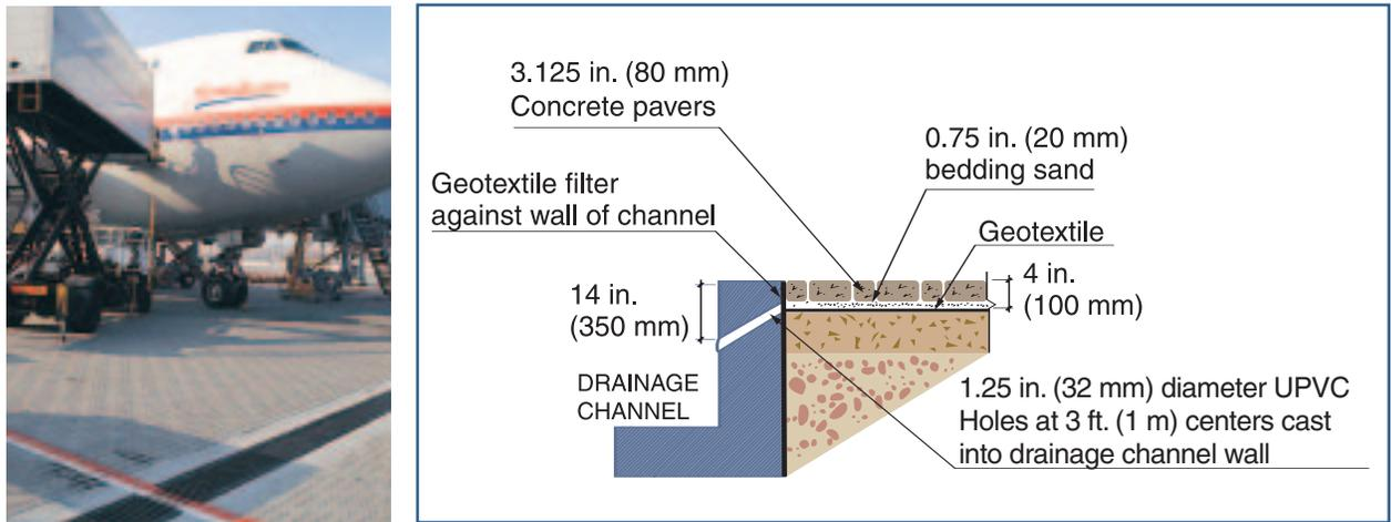
the pavement, the drain holes dissipate excess water in the bedding sand, thereby reducing the chance of pore pressure build-up and sand loss through the joints. To ensure that the bedding sand was not washed away through the weep holes, the geotextile continued up the face of the drainage channels to  $\frac{3}{8}$  in. (10 mm) below the surface.
