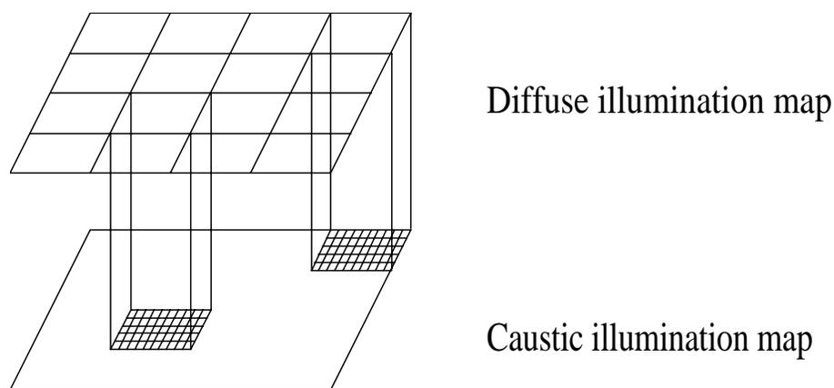
Figure 3: The figure shows how the illumination map is divided into two levels, one for caustics and one for "diffuse" illumination.
