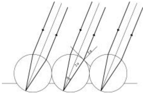
Fig. 10 Retro-reflective surface densely covered with microscopic beads with about 50 micrometer diameter. Ideally, refractive index should be 2.
