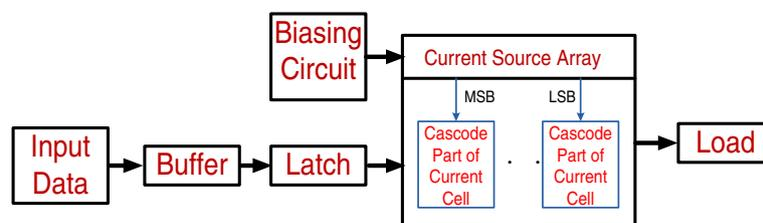
Figure 1 Overall block diagram of the proposed DAC.
