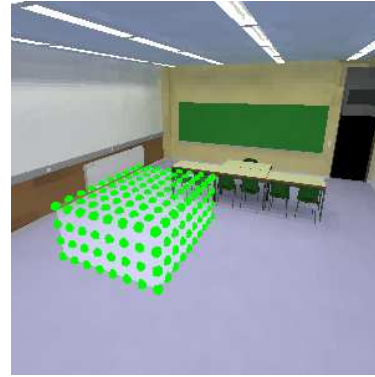
Figure 6: The positions of the camera are selected over the semi-transparent polyhedron that bounds the walking region.
