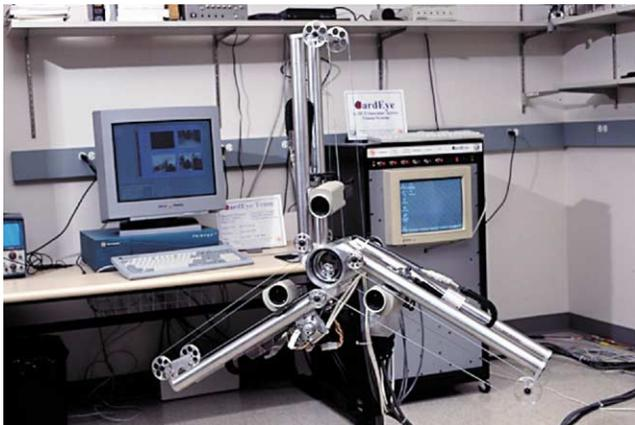
Fig. 1. CardEye trinocular active vision system: From left to right, the trinocular head and the control circuitry cabinet.
