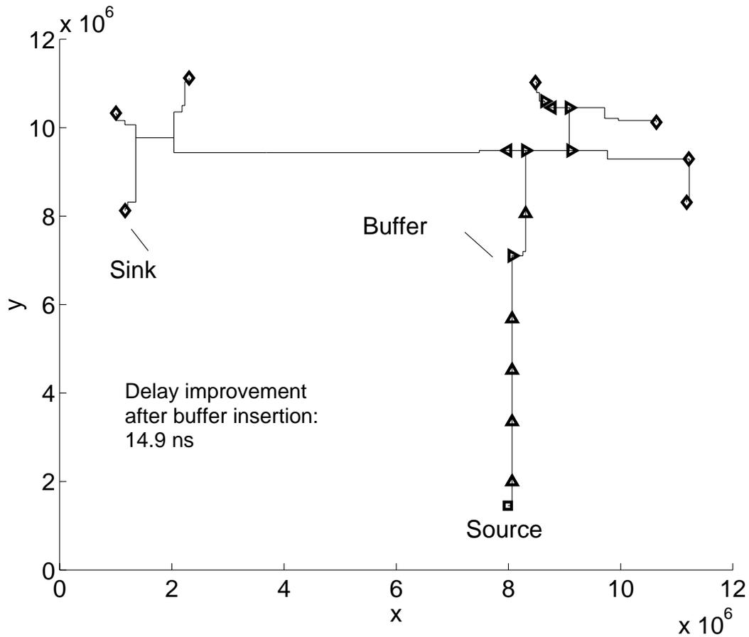
Fig. 1. One 7-sink net extracted from an ASIC chip. Before buffer insertion, the slack of the net is  $-13.9\text{ ns}$ . After 12 buffers inserted, the slack becomes  $1.0\text{ ns}$ . The delay improvement is  $14.9\text{ ns}$ .
