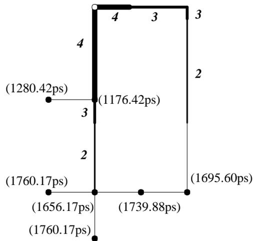
Fig. 34. Example of our algorithm applied to a non-tree topology. The white node is source, black nodes are sinks, and grey nodes are new sink nodes generated from splitting an edge.
