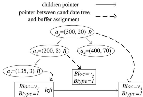
Fig. 13. Four candidates with their buffer types and locations:  $\alpha_4$  has no buffer,  $\alpha_3$  has one buffer at  $v_3$ ,  $\alpha_2$  has one buffer at  $v_2$ , and  $\alpha_1$  consists of  $\alpha_3$  and a buffer at  $v_1$  as shown in Fig. 10.
