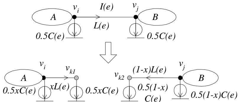
Fig. 31. Edge cutting. If  $0 \leq I(e) \leq 0.5C(e)$ , edge  $e = (v_i, v_j)$  is cut into two edges  $(v_i, v_{k1})$  and  $(v_{k2}, v_j)$ , such that the Elmore delay for every node in the entire circuit is unchanged.  $A$  is the part of the circuit adjacent to  $v_i$ , and  $B$  is the part of the circuit adjacent to  $v_j$ . Symbol  $\underline{\oplus}$  represents a current source.
