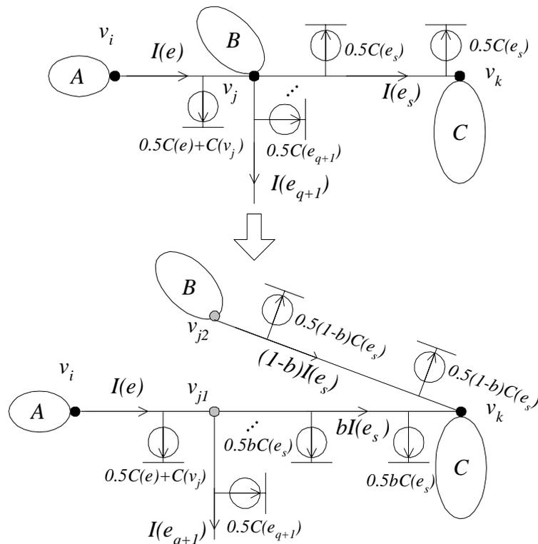
Fig. 33. Edge splitting. If  $I(e) > 0.5C(e) + C(v_j)$ , edge  $e_s = (v_j, v_k)$  is splitted into two edges  $e_{s1} = (v_{j1}, v_k)$  and  $e_{s2} = (v_{j2}, v_k)$ .  $A$  is the part of the circuit adjacent to node  $v_i$ .  $B$  is the part of the circuit adjacent to node  $v_j$  including edges  $e_2, \dots, e_q, e_{s+1}, \dots, e_d$ .  $C$  is the part of the circuit adjacent node  $v_k$ .
