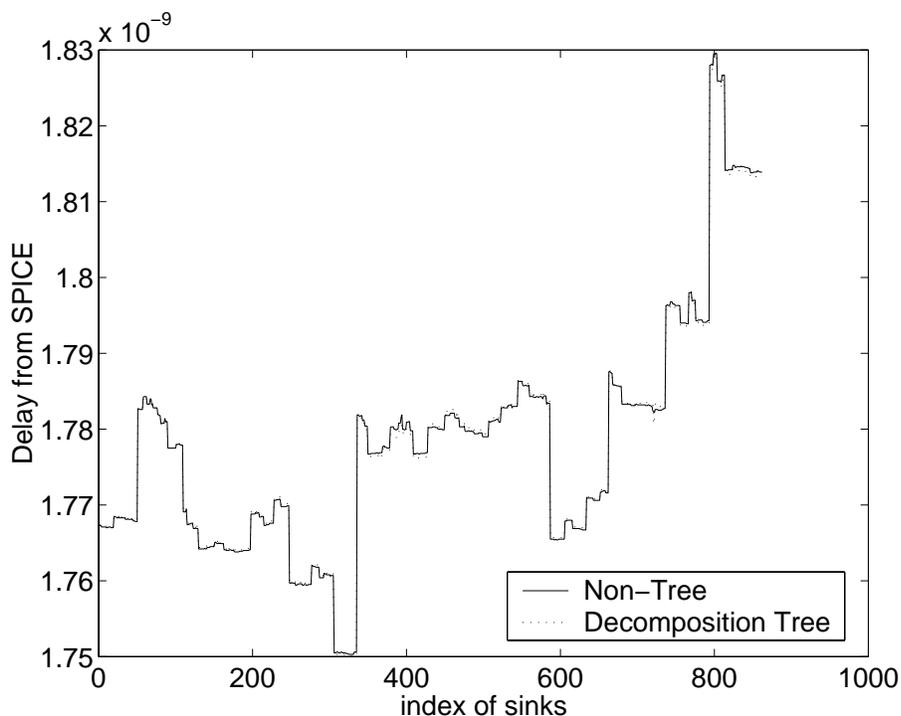
Fig. 35. SPICE delay for all sinks in original non-tree topology and decomposed tree tree topology
