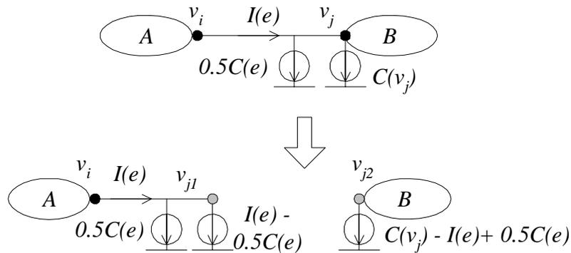
Fig. 32. Node splitting. If  $0.5C(e) < I(e) \leq 0.5C(e) + C(v_j)$ , node  $v_j$  is splitted to two nodes  $v_{j1}$  and  $v_{j2}$ , such that the Elmore delay at every node in the entire circuit is unchanged.  $A$  is the part of the circuit adjacent to node  $v_i$ , and  $B$  is the part of the circuit adjacent to node  $v_j$ .
