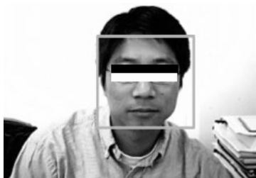
Fig.3. Detecting a human face with a Haar-like feature
