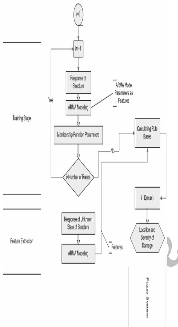
**Figure ( 2):** Flowchart of proposed damage detection method.
