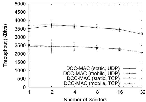
Fig. 13. Random mobile network: Surface area of  $20\text{m} \times 20\text{m}$  and mobility according to the random waypoint model. On the x-axis is given the number of nodes in the network and on the y-axis is the average rate per user.
