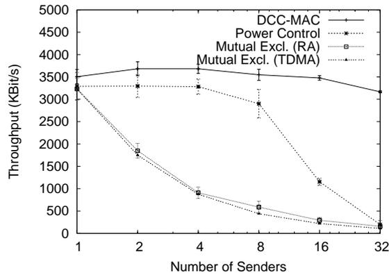
Fig. 11. Random scenario with nodes placed on  $20\text{m} \times 20\text{m}$  square. The number of nodes is given on x-axis, and the average rate is given on the y-axis.
