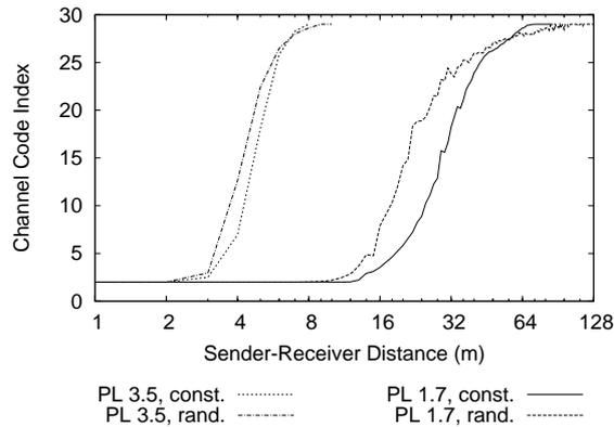
Fig. 7. UWB signal propagation for LOS and NLOS over distances of 1m-100m. The lower the SINR due to the sender-receiver distance, the higher the index of the chosen channel code. Non-line-of-sight communication is possible for up to 10m, line-of-sight communication for up to 60m.
