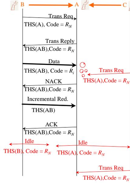
Fig. 5. Private MAC:  $B$  sends to  $A$ ,  $C$  attempts to send to  $A$  and is deferred. No collision occurs because  $B$  and  $C$  use different Time Hopping Sequences.
