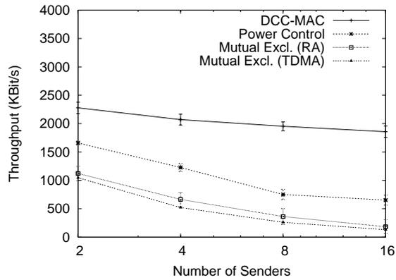
Fig. 9. Near-far scenario with a link length of 20m. We show average rate per user vs. number of (mutually interfering) senders.
