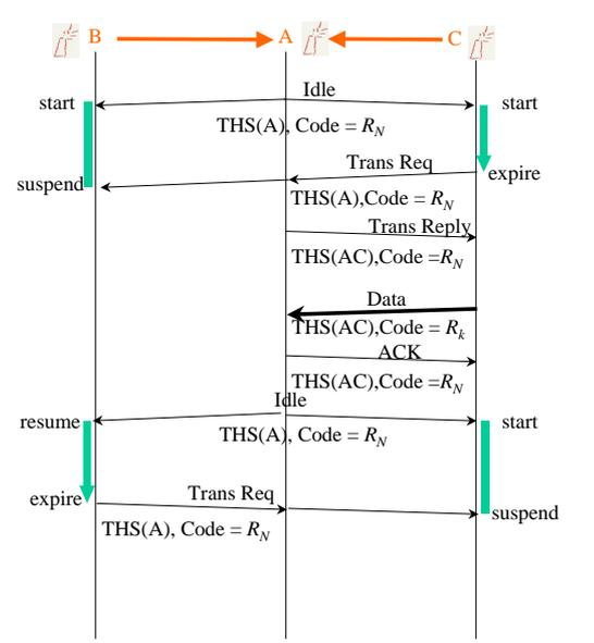
Fig. 6. Private MAC, showing state of backoff timer.  $B$  and  $C$  compete for sending to  $A$ .  $C$  initially draws a shorter backoff timer and gains access to  $A$ .
