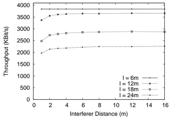
Fig. 8. Near-far scenario with 2 senders (i.e., 1 interferer) and for different sender-receiver distances ( $l$ ). We show average rate per user vs. distance to the interferer. Only for very close interferers, DCC-MAC throughput decreases slightly.
