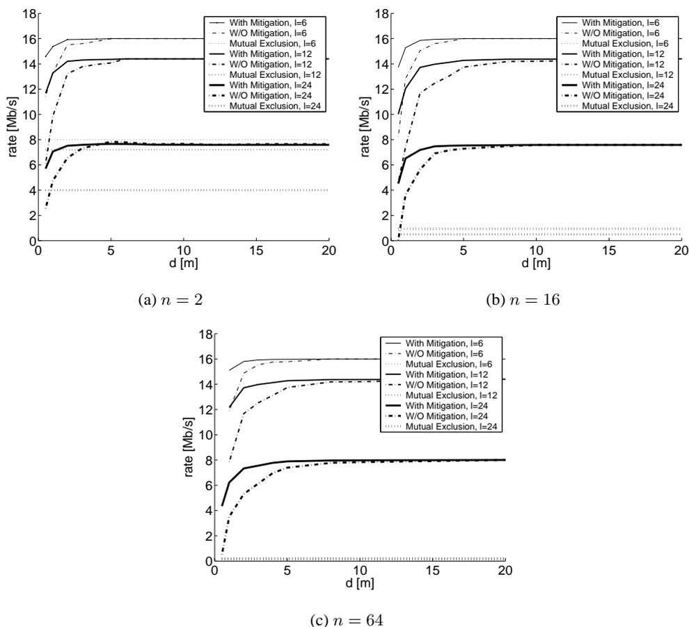
Fig. 3. Rate achieved in the multiple interference scenario, for All-at-once and mutual exclusion, and various link lengths  $l$ , versus distance to  $d$  from the interferer to the destination, for various numbers  $n$  of interfering links.
