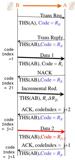
Fig. 4. Dynamic Channel Coding: text above an arrow refers to the content of the message, text below gives the message's THS and channel code.
