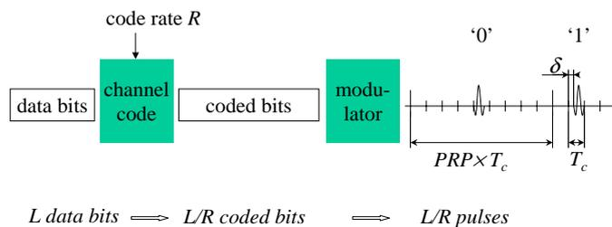
Fig. 1. Model of Ultra Wide Band used in this paper
