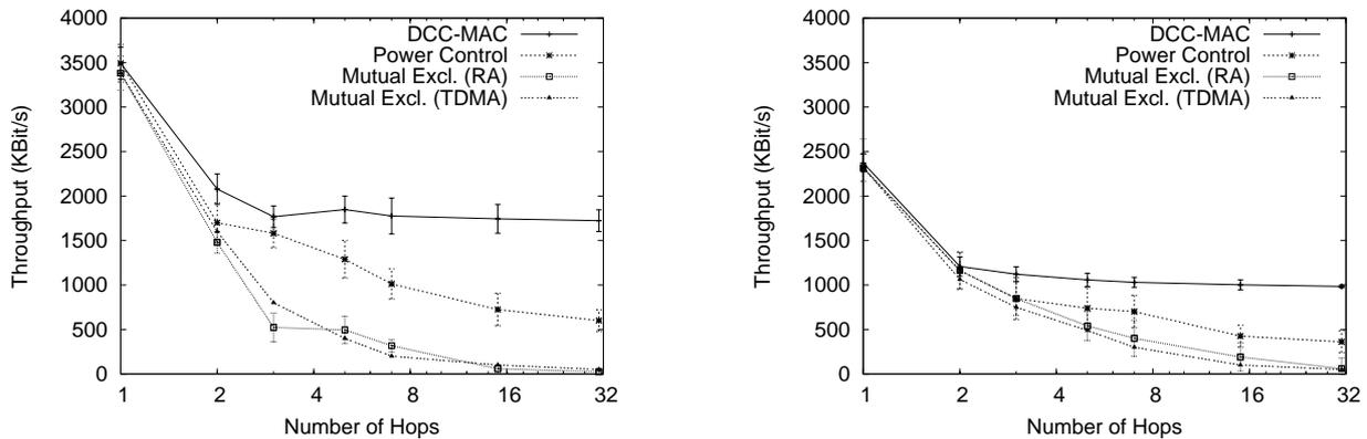
Fig. 10. Throughput on the multi-hop network for UDP (left graph) and TCP (right graph). We show throughput vs. number of hops. There is almost no drop in throughput for the DCC-MAC as the number of hops increases.
